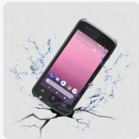
Rugged Design (1.5m drop test IP67 whole unit)
